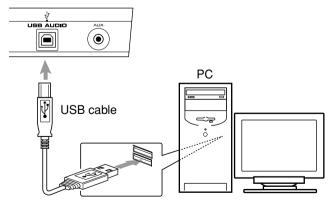
• Use "USB series A plug to B plug" cable when connecting.
