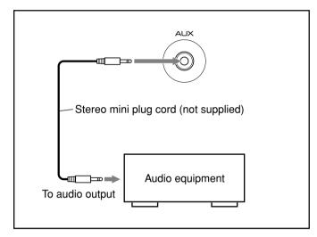
For playing the other equipment through this unit, connect between the audio output jack on the other equipment and AUX jack on the front of the unit by using a stereo mini plug cord (not supplied).
